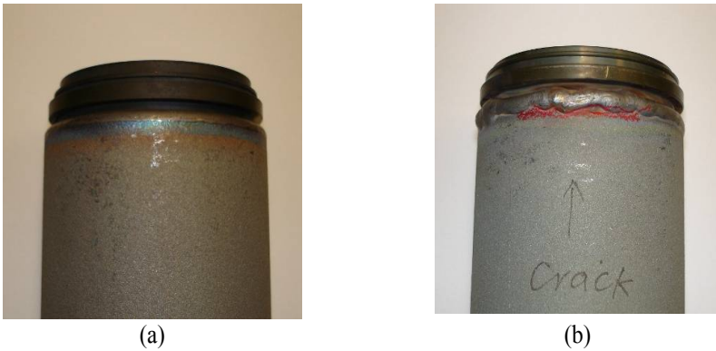
FIGURE 8. (a) A defect free part and (b) a cracked filter. Note the difference in the weld.
